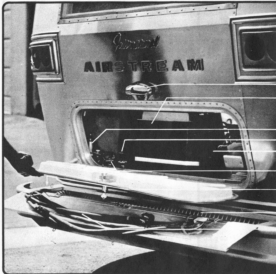
This photograph shows the "One-Stop Service Center" This feature gives quick access for "hook-up" and service of most of the self-contained utilities in your trailer. Details of the utility systems are discussed in chapters 6 through 9.
